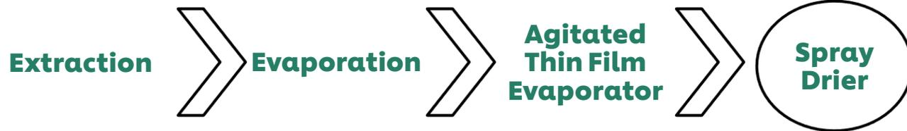
**Liquor at 10.6% concentration**      **Liquor concentration increased to 50%**      **Liquor concentration increased to 60%**      **Liquor sprayed to produce IC powder**
